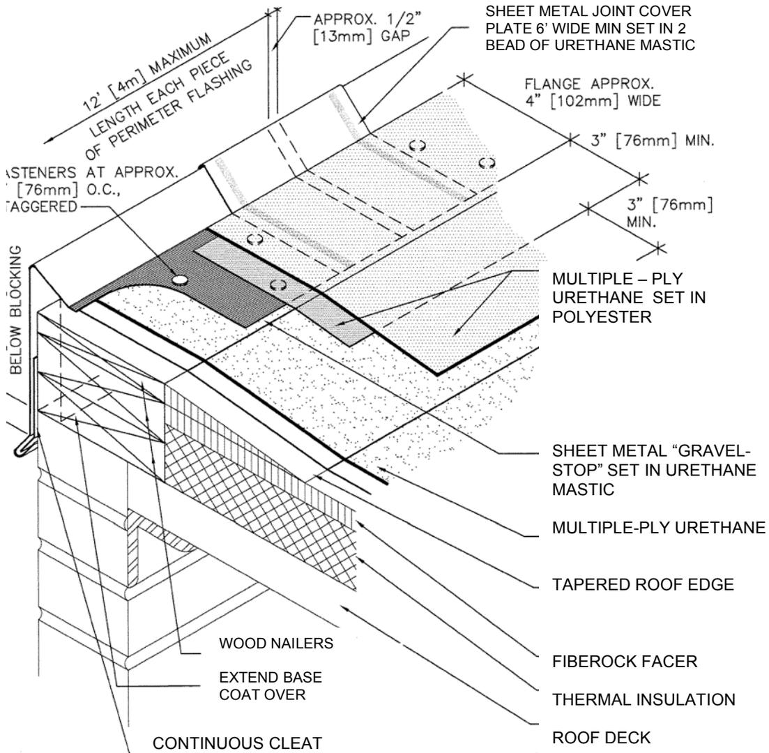
**POLYMER BUILT UP ROOFING**
