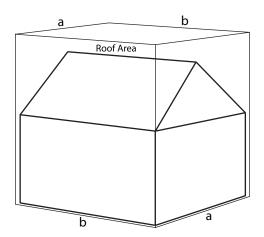
The catchment area of the roof is a simple calculation of width x length of the house. To find out how much rain will be collected, take the area of the roof, multiply by the annual rainfall amount, then multiply by .5618 to arrive at the average number of gallons yearly.
